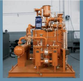
The machine requires lubricating oil even after it has been ordered to stop or after an emergency block, to ensure safe stoppage down to 0 revolutions of the shaft.
