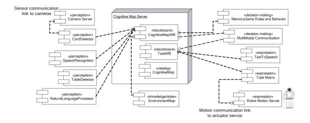
Fig. 2. Overview of the Cognitive Map robot architecture: Representative components depicted showing connectivity to the central Cognitive Map server. Component types are labeled above name. Arrow directions depict dependencies on various interfaces (not message directions).
