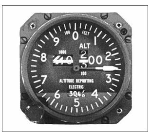
Figure 1-8. Drum-pointer altimeter
