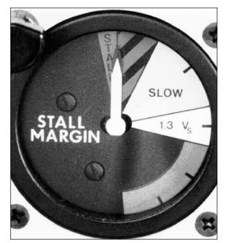
Figure 1-4. Angle of attack indicator
