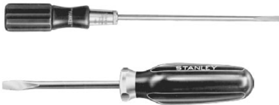
Figure 2.12 Electrician's screwdrivers ( top ) are designed for precision work; standard screwdrivers are used on heavier jobs ( bottom ). (Stanley Works)
