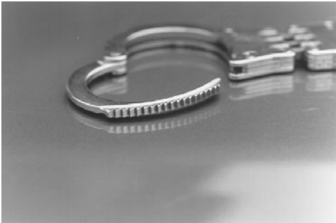
Figure 17.12 The ratchet of a cuff has a row of teeth that are angled in a direction to allow the cuff to close freely but not to open without a key.
