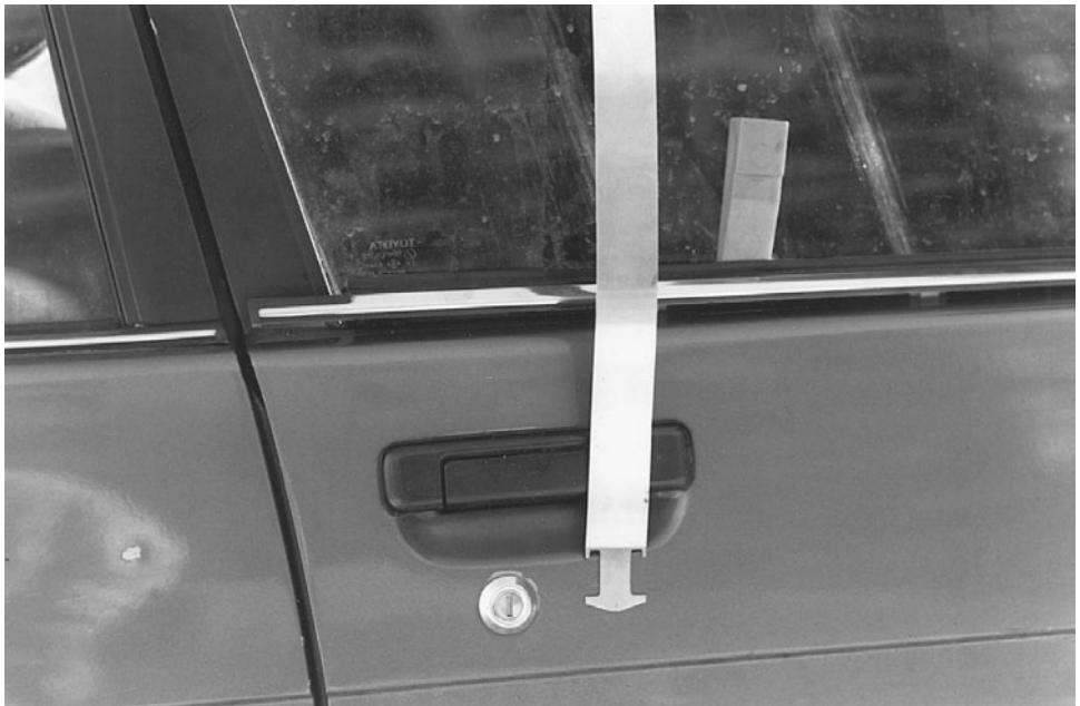
Figure 16.1 A slim jim shown outside of a door.
