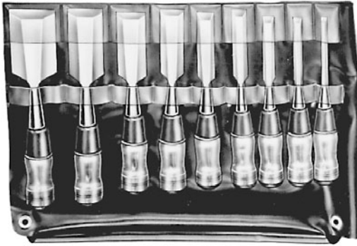
Figure 2.39 Wood chisels of various sizes are needed when installing locks and other hardware on wood doors. ( Stanley Works. )
