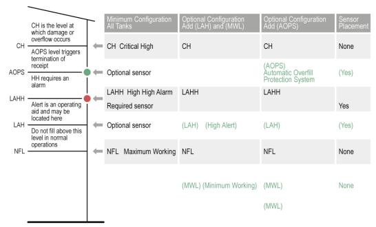
Notes: 1. It is recommended that a Minimum Working Level (MWL) be established for all tanks.
