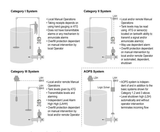
Figure 2: Definition of Overfill Protection System Categories
