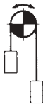
Figure 4.3 Hanging Transmission Where Conveyed Objects Are Lifted or Suspended at the End of Chains
