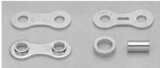
Figure 1.17 Bushingless Bicycle Chain Components
