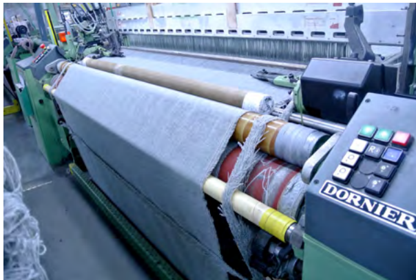
An example of a simple weave produced on a dobby loom
