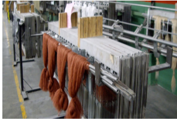
This shows the harnesses that move up and down during weaving to create the pattern.
