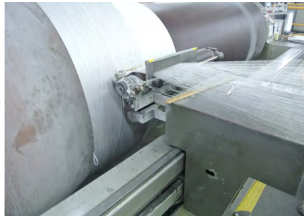
A close-up of the warping drum on which the yarns are wound and built up in sections. The warping drum spins to wind the yarn around it.
