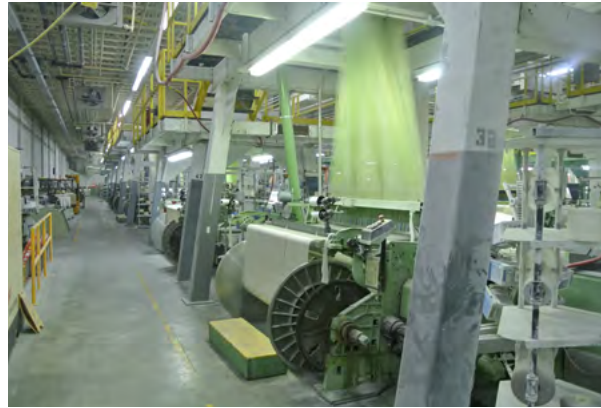
You can immediately spot a Jacquard loom because of the harnesses extending upward to the controller.
