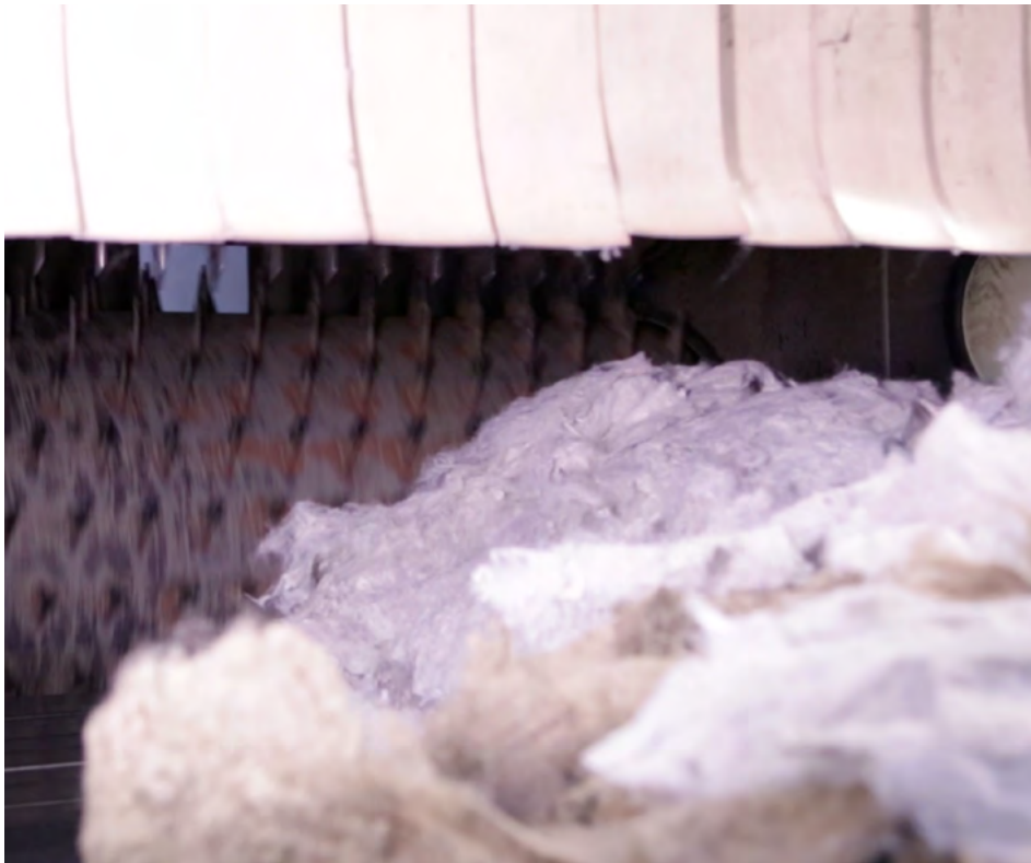
Fiber being fluffed after being compressed in the dye cakes
