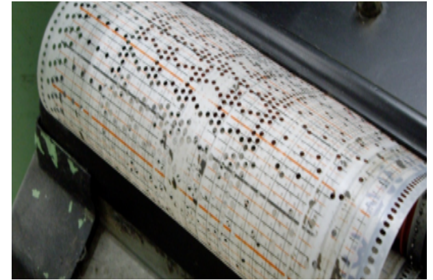
Similar to a player piano, the harnesses are controlled by a mylar card
