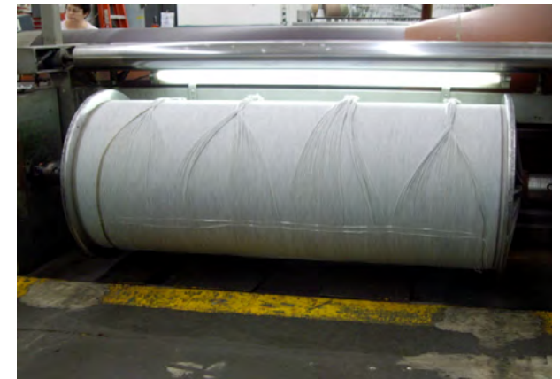
A completed warp, also showing it transferred from the tapered warper to the beamer, which looks like a giant spool. From here it will be transported to the loom.
