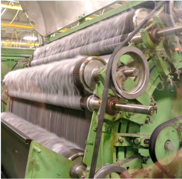
These drums are covered in wire pins. The drums spin to arrange the fibers in the same direction.
