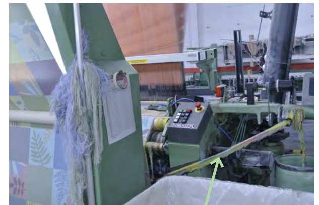
Here you can see the selvage being removed
