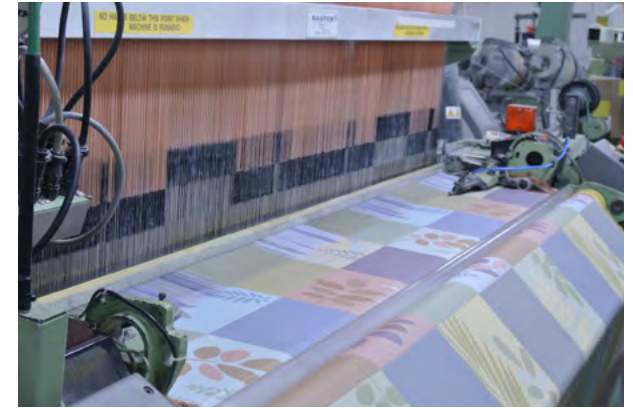
Different sections of the harnesses are being lifted to create the intricate pattern
