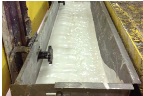
Backcoating, with latex added to the blade
