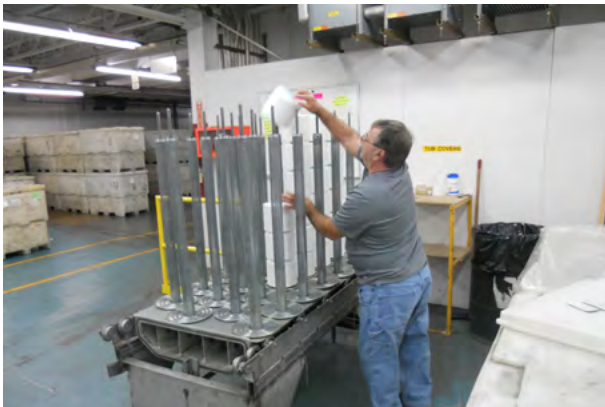
The yarn is wound on a perforated tube called a package and placed together on a rack.
