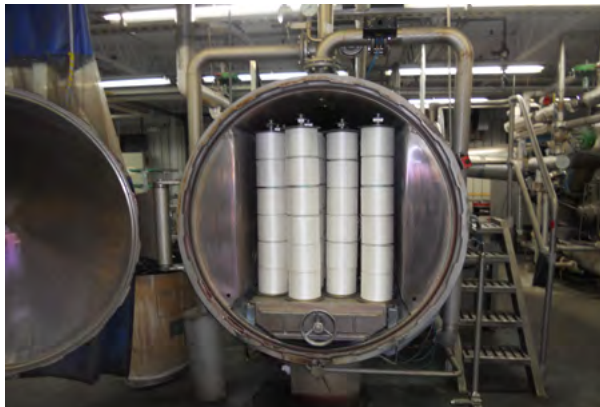
The white yarn is placed into the dyeing machine.
