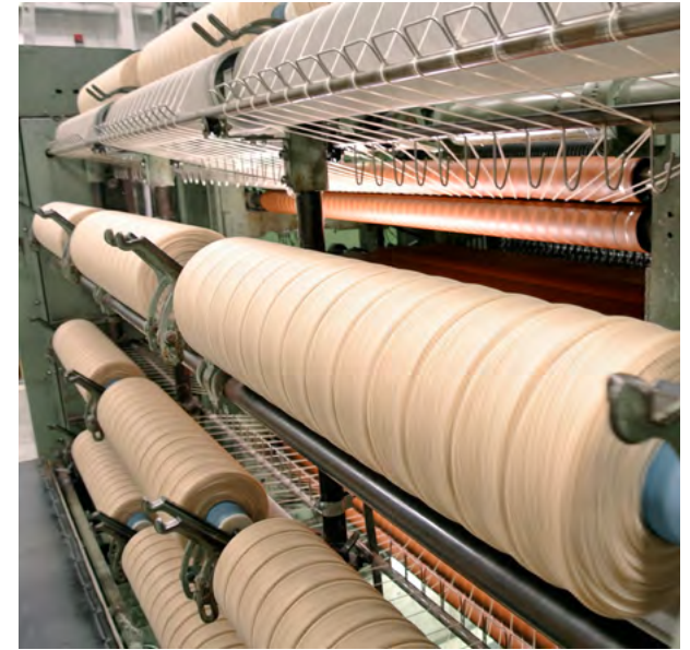
At the end of the carding machine, the fibers are slit into narrow widths and spun onto a spool. This is sliver.
