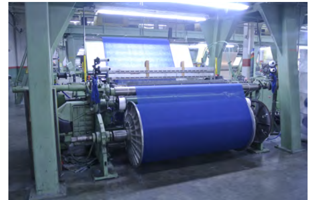
Here you can see the warp beam hooked up to the loom
