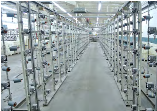
This shows the creel, which holds the spools of yard that are wound onto the warping drum.
