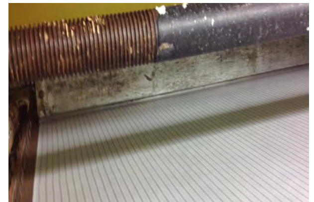
Backcoated fabric exiting the blade
