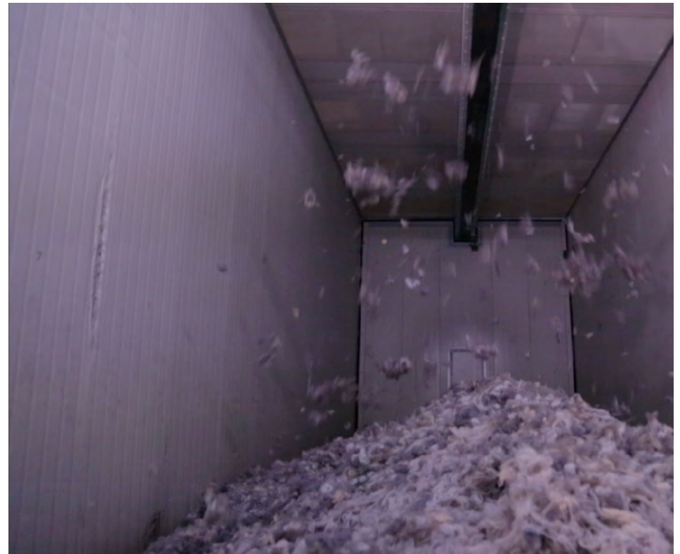
Fiber being blown in order to mix it consistently
