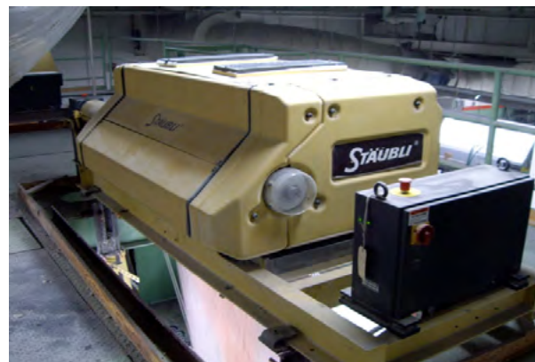
The computer that controls the harnesses of a Jacquard loom
