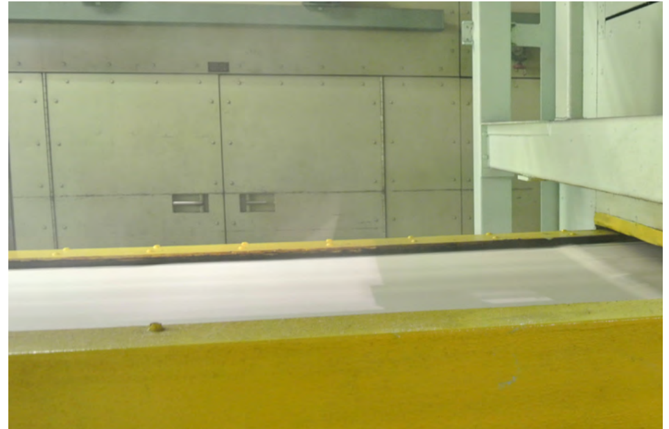
Fabric coming through the oven after being treated
