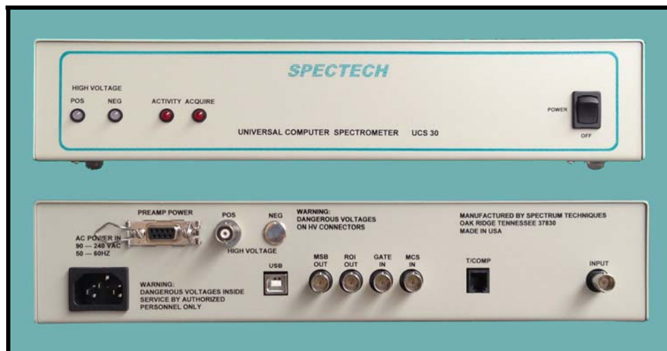
Figure 17. Front and back panels of the multichannel analyzer used in this experiment, the Spectrum Techniques Model UCS-30 Universal Computer Spectrometer.
