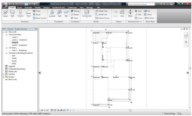
Figure 7: A Linked Drawing from AutoCAD
