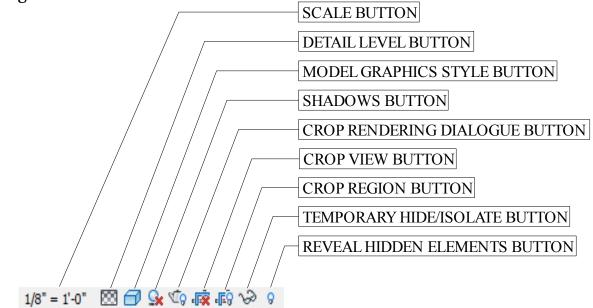
Figure 2: The View Control Bar Buttons
