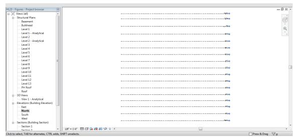
Figure 5: Created Levels For a Structure
