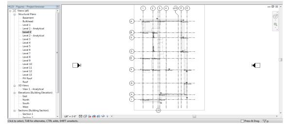
Figure 11: Created Grid Lines for a Structure
