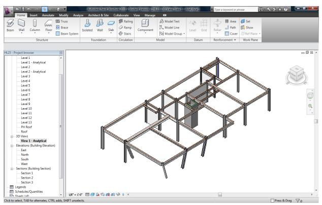
the **Place Beam > On Grid Lines** tab to create the displayed beams.
