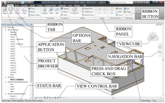
Figure 1: The Revit User Interface and Toolbars
