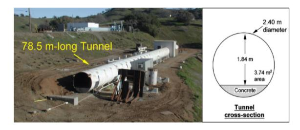
Ref: Groethe et al., 2007  $1/5^{th}$  scaled real tunnel Length×Height =  $1.84 \times 79.5m$ 9.5-30% vol. H<sub>2</sub> experiments  $0.32 - 1.0 \text{ kg H}_2$
