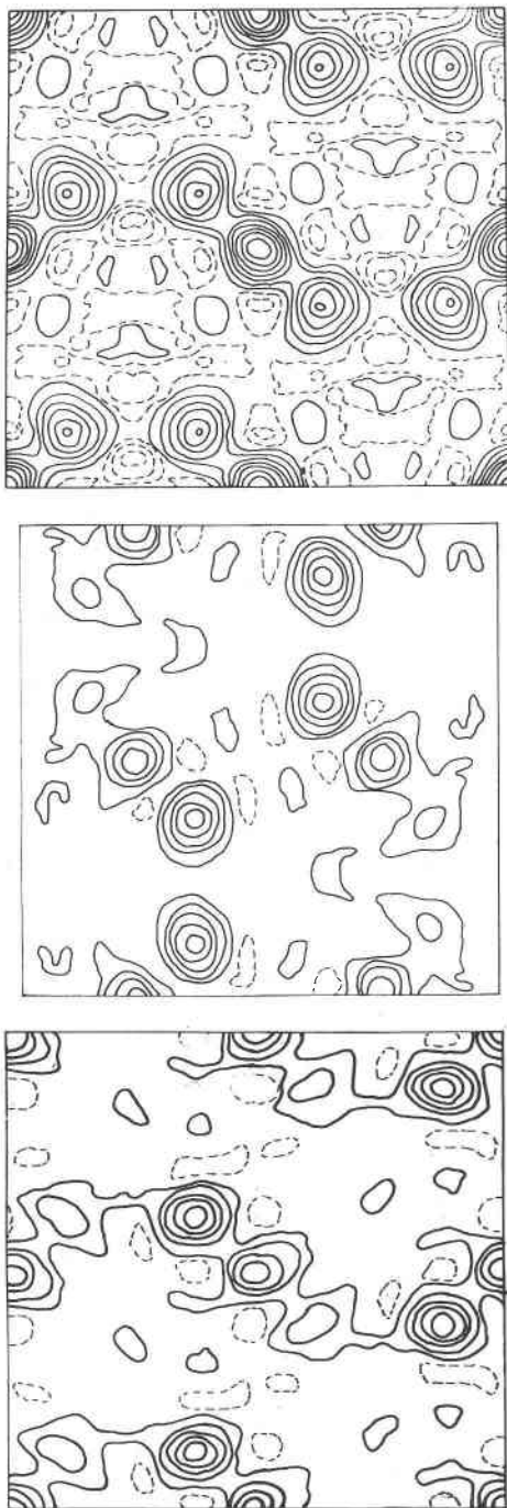
FIG. 3. Electron density projections of disordered (3a) and ordered cobaltite (3b, 3c). The contours are drawn with an arbitrary interval. The first solid contour is at height zero. Figure 3a is projected onto (001). Figures 3b and 3c are projected onto (001) and (010) respectively.
