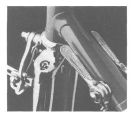
Figure 1-11: This microfusione (cast) fork crown carries the logo of its builder—Gios-Torino.
