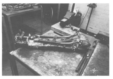
**Figure 1-5:** Fork jigs are usually fairly simple and variations between builders are slight. This is a jig used by Bob Jackson (chapter 5). The fork has just been brazed and therefore has a very rough appearance.
