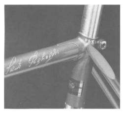
Figure 1-16: Note the beefy-looking, 16-mm. semi-wrap stay used on this 58-cm. track bicycle. Pogliaghi (see chapter 16) adds a personal touch to his bicycles with a transfer of his signature on the top tube.
