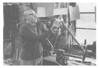
Figure 8-2: Jack Taylor fits the bottom bracket on a custom tandem.
