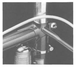
Figure 1-15: This semi-wrap style is usually accomplished with a "plug." This is a 12-mm. stay such as found on a 49-cm. Colnago road frame.
