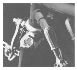
Figure 1-9: This cutout is so famous that it immediately identifies the builder as Ernesto Colnago. In this case, the clover leaf also appears on the semi-sloping fork crown.
