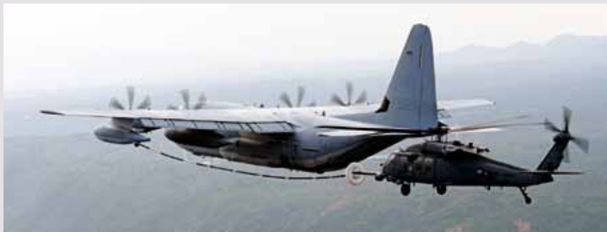
Figure 4. An HH-60G-Pave Hawk helicopter from the 33rd Rescue Squadron (RQS) receives fuel from a KC-130J during a 3-day intensive air refueling course at Kadena Air Base, Japan. The KC-130J, which performs air-refueling missions, is a specialized version of the C-130J, a medium-range, tactical aircraft and the newest upgrade to the C-130 fleet. U.S. Air Force photo by SSgt Chrissy Best.
