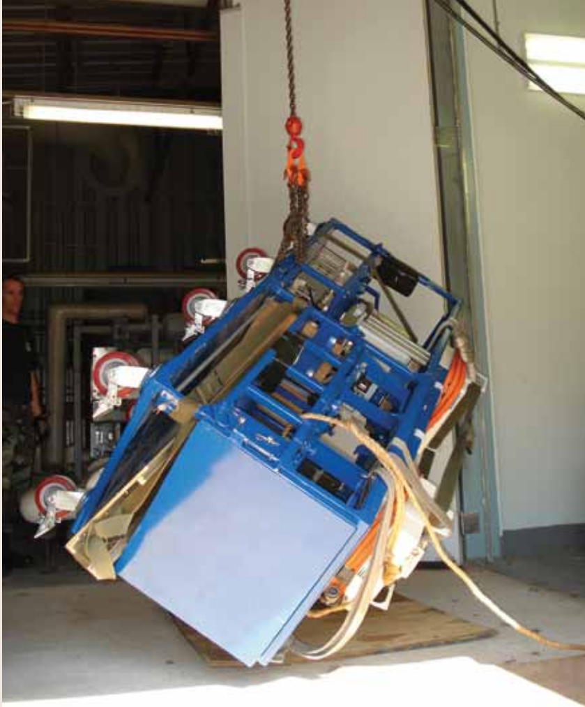
FIGURE 10. VIEW OF SUT NO. 1 DURING HANG TEST
