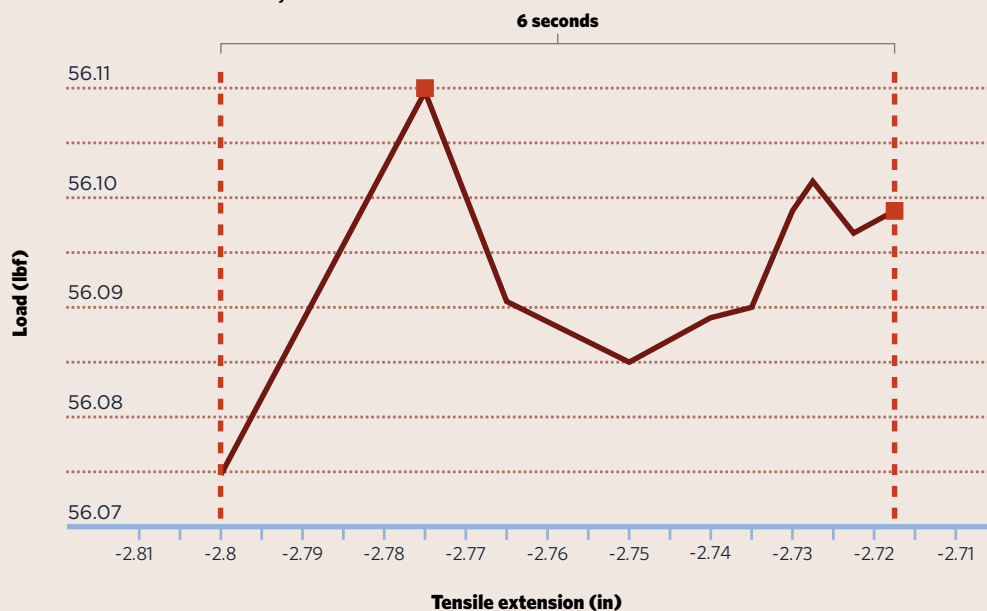
FIGURE 6. EUT NO. 1—LOAD CURVE MEASURED DURING TENSILE TESTING, ORIENTATION NO. 2
