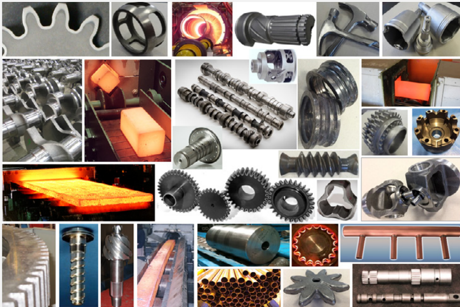
Fig. 2: Variety of workpiece geometries that routinely apply induction heating (Courtesy of Inductoheat Inc.)
