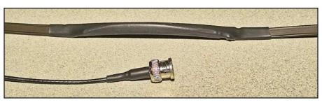
Figure 5 — The  $\lambda/4$  UHF decoupling stub made of RG-174A, covered with heat shrink tubing. This is shown next to the BNC connector that goes to the transceiver.
