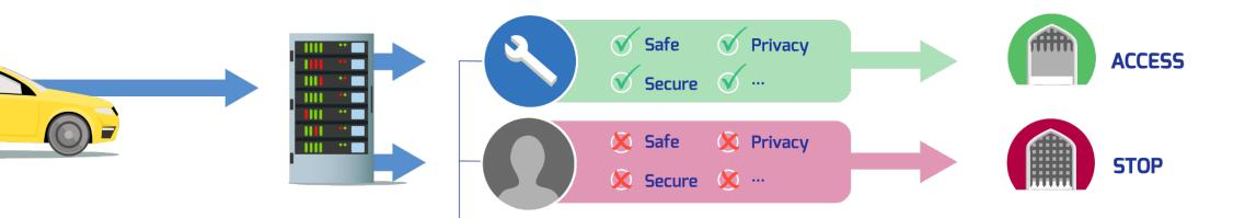
Relevant vehicle data are communicated by the manufacturer to an off-board facility Service providers can then access vehicle data through off-board means, rather than having direct access to the vehicle in an uncontrolled way The off-board facility acts as a gatekeeper, minimising safety, security and liability risks
