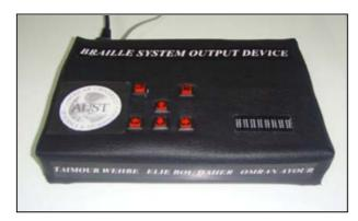
Figure 4. The multi-lingual Braille system output device with audio enhancement developed in this study.
