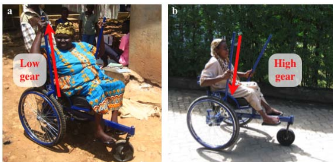
Figure 1 MOVING HAND POSITION TO CHANGE MECHANICAL ADVANTAGE a) Placing hands high on the levers generates high torque and an effective low gear. b) Placing hands low on the levers creates high angular velocity in the drivetrain and an effective high gear.
