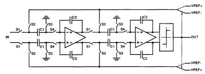
Fig. 10. Second-order  $\Sigma\Delta$  modulator implementation.
