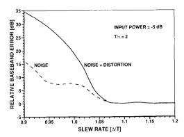
Fig. 7. Simulated influence of integrator output slew rate on baseband quantization noise.
