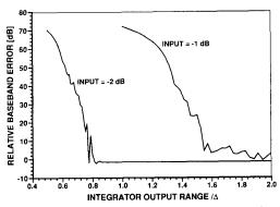
Fig. 4. Simulated influence of integrator output range on baseband quantization noise for input sinusoids 1 and 2 dB below overload.
