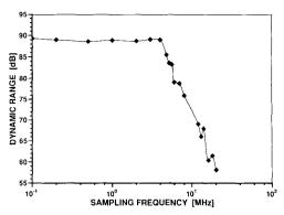
Fig. 14. Maximum operating frequency.
