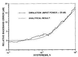
Fig. 9. Influence of comparator hysteresis on baseband quantization noise.
