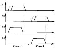
Fig. 11. Clock diagram for second-order  $\Sigma\Delta$  modulator.
