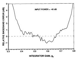
Fig. 5. Simulated influence of variations in integrator gain on baseband quantization noise.
