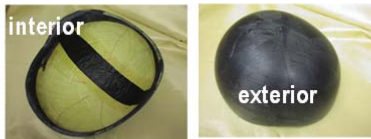
Figure 15. Integrally stiffened KM2-polyolefin shell.
