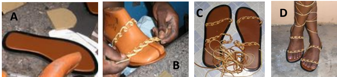
Fig. 4A, B, C & D: Forming the sole, measuring, fixing the top and the completed sandals
