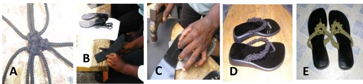
Fig. 3A, B, C, D & E: Making the top, the sole and the pair of the slippers
