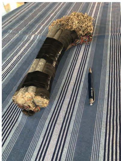
An artifact from Trinity Church, 1,486 conductors (plus positive and negative DC leads) (photo credit: John Bishop)
