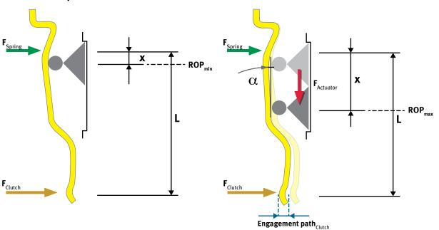
The pre-tension force of the pressure spring  $[F_{\text{Spring}}]$  in the return spring and the leverage ratio [x/(L-x)] resulting from the position [x] of the sled determine the engagement force of the clutch  $[F_{\text{Clutch}}]$ .
