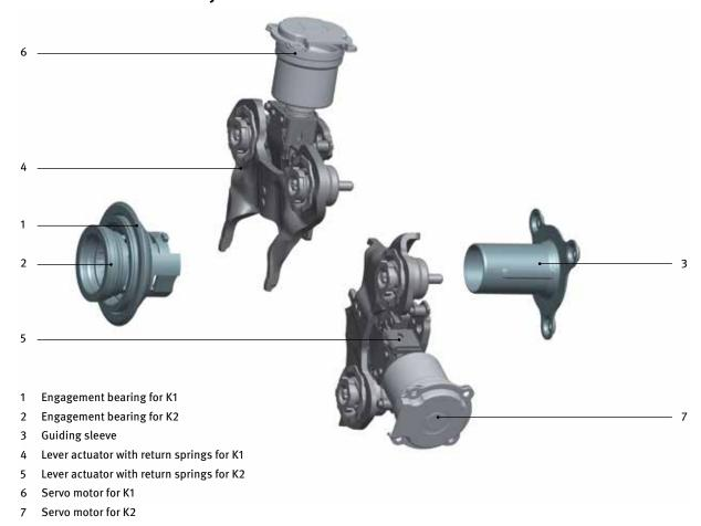
With previous manual transmissions with single disc clutch, the clutch is closed when idling. It is opened by pressing on the clutch pedal, thus disconnecting the transmission of power. This takes place via the "release system".
