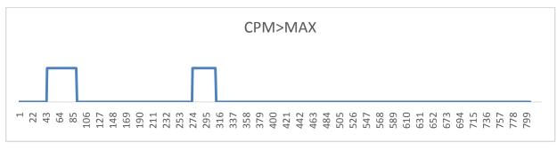
*Figure 8:* Comparison of days of the project where the resources of the CPM method are greater than the maximum amount of resources.
