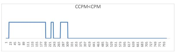
Figure 7: Comparison of days when resources of the CCPM method are less than CPM
