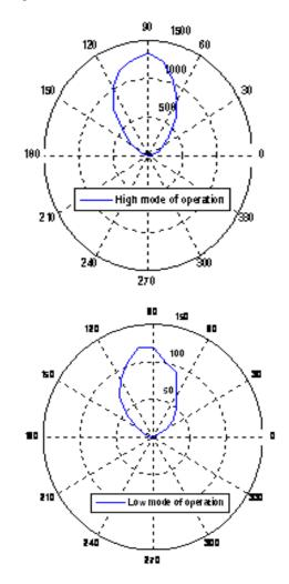
Figure 6: Radiation pattern of output light intensity of LED lamp
