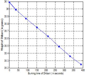
Figure 2: Rate of kerosene fuel consumption by Dhibari
