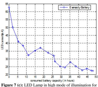
Figure 7 (c): LED Lamp in high mode of illumination for Geep and Eveready batteryFigure 7: Variation in LED current with running hours of battery supplied from local manufacturer
