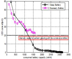
**Figure 8(b):** LED lamp in high mode of illumination **Figure 8:** Discharge curves of low cost battery supplied from local manufacturer with respect to LED current (a) Panasonic, Nippo, Eveready and Geep batteries used in low mode of illumination of LED lamp (b) Geep and Eveready battery used in high mode of illumination of LED lamp.
