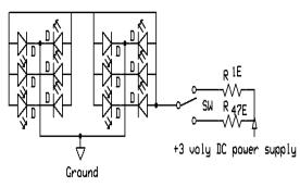
Figure 4(b): Circuit diagram of LED lamp
