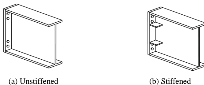
Figure 1.2. Flush end-plate connections
