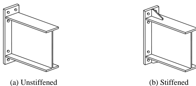
Figure 1.3. Extended end-plate connections
