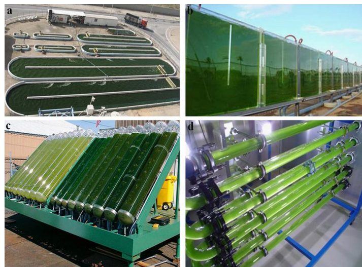
Figure 1. PBR designs: a- open ponds, b- flat panels, c- outdoor tubular PBR, d- indoor tubular PBR [50].
