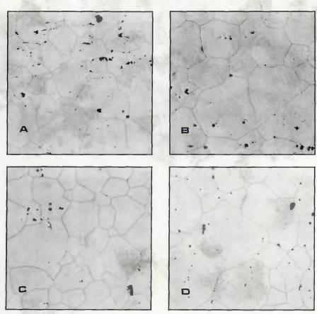
Fig. 5 – Typical microstructures of age hardened Alloy 718. A-0 h at 650°C; B-1 h at 650°C; C-10 h at 650°C; D-25 h at 650°C. Grain size 60  $\mu$ m
