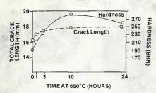
Fig. 9 – A comparison of the change in microfissuring susceptibility with the change in hardness during age hardening. Grain size 60 μm
