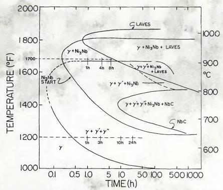
Fig. 1 - Transformation diagram for Inconel 718 showing heat treatment schedule
