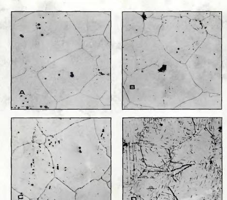
Fig. 4 — Typical microstructures of solution annealed Alloy 718. A — 0 h at  $927^{\circ}C$ ; B — 1 h at  $927^{\circ}C$ ; C — 4 h at  $927^{\circ}C$ ; D — 8 h at  $927^{\circ}C$ . Grain size  $200~\mu m$
