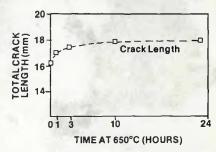
Fig. 7 – The change in microfissuring susceptibility during aging at 650°C. Grain size 60 μm
