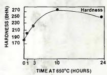
Fig. 3 – The rate of hardening during aging at 650°C. Grain size 60 μm
