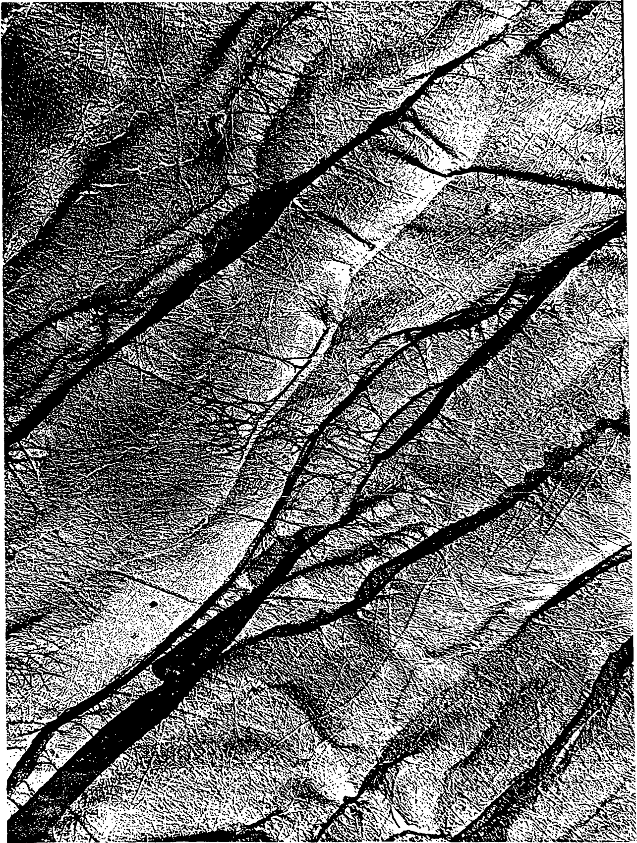
Figure 23. 9% KOH-3% H_3BO_3 -Extracted Holocellulose Fiber 30,000 X
