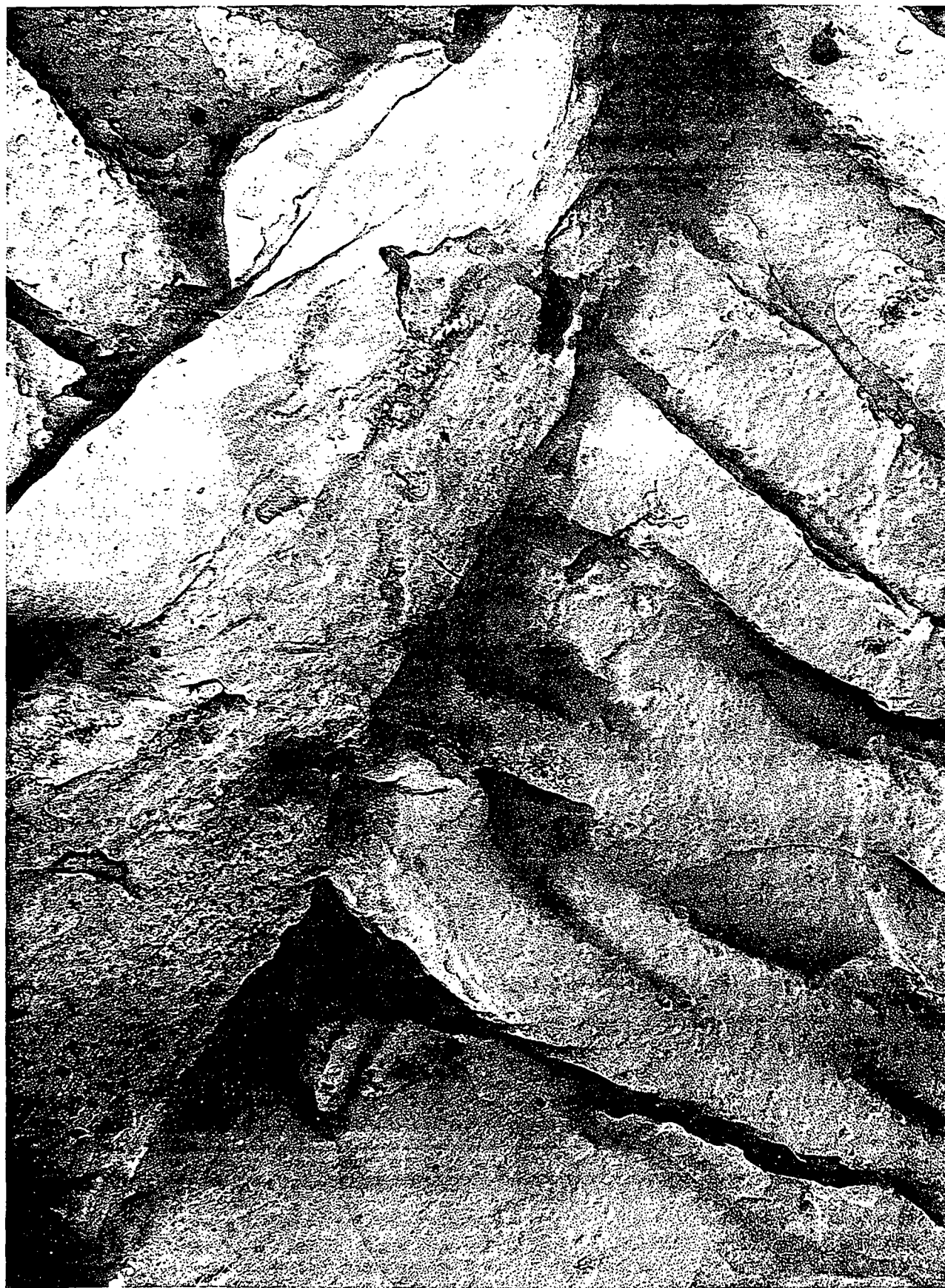
Figure 20. Nonextracted Holocellulose Fiber 43,000 X
