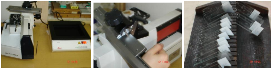
Figure 2.18. Sliding microtome that was utilized for taking sections from samples (Samples were collected by microscope slides).
