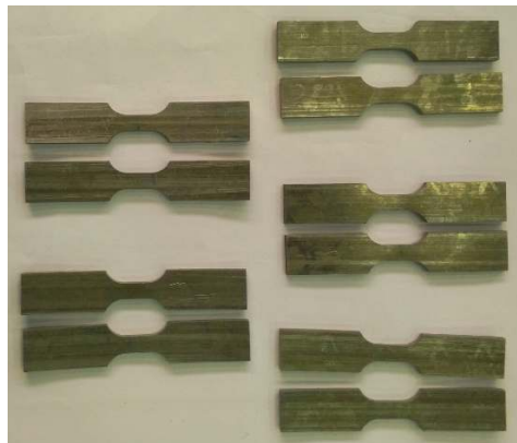
Figure 2. The samples prepared for the uniaxial tensile test.
