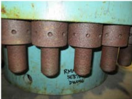
Figure 12- Corroded motor cover studs (left) and close up of stud (right)
