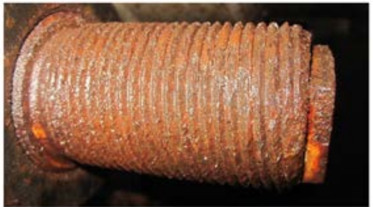
Figure 12- Corroded motor cover studs (left) and close up of stud (right)
