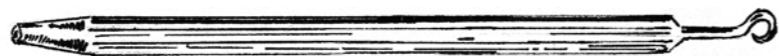
SIMPLE HALF-HITCH TOOL, IN THIS CASE WITH A DUBBING TWIST HOOK ON THE OTHER END
