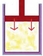
THE PISTON IS COMPRESSED SO THAT THERE ARE NO HEAT EXCHANGE.
