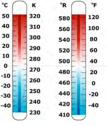
A *thermometer* is a device that is used to measure temperature. A thermometer works due to a physical change in a material as a function of temperature and a means of converting the physical change into a temperature.
