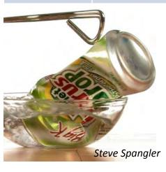
In the can crush experiment, the barometric pressure outside the can is much greater than the pressure inside the can. The can is crushed (changes its volume) to equalize the external and internal pressure.
