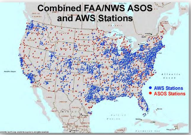
ASOS = Automated Surface Observing Station AWS = Automated Weather Station
