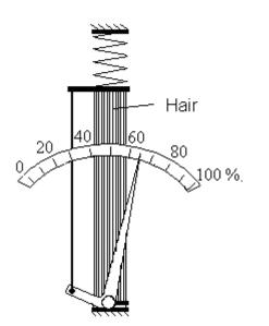
**Hair hygrometer.** Human and animal hair changes its length as a function of humidity. A hair hygrometer is a mechanical device that magnifies the change in the hair and is indicated by a dial.
