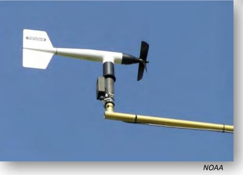
An *aerovane* can simultaneously measure wind direction and speed.
