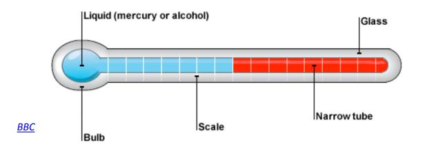
At 20 °C, the volume of mercury expands 0.02% per degree.
