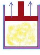
THE PISTON IS EXPANDED IN A WAY THAT THERE ARE NO HEAT EXCHANGE WITH THE ENVIRONMENT. AS A CONSEQUENCE, TEMPERATURE AND INTERNAL ENERGY OF THE SYSTEM DECREASE.
