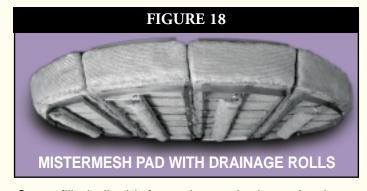
Once filled, liquid from the pad above is drawn through surface tension to the coils, thereby establishing distinct regions for liquid drainage and liquid collection in the upstream layers. Figure 18 compares the pressure drop and flooding point of both conventional and MisterMesh® Mist Eliminators.
