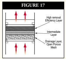
between the collection and drainage zones. Figure 17 illustrates a Multilayer mist eliminator.
