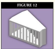
As the fluid flows axially towards the shell opposite of the inlet nozzle, liquids are captured by specially placed blades. This design is superior because it allows the escape of liquids over a much greater
