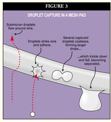
For fogs in which the bulk of the droplets are characterized with submicron diameters, the energy to bring about the collision with the target is derived from Brownian Diffusion, the random motion of fine liquid
