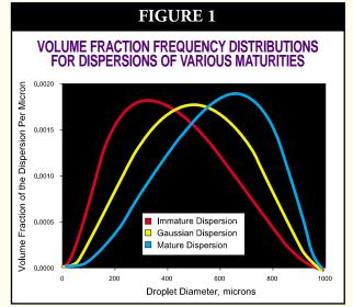
In practice, designers or engineers do not quantify or measure droplet size distributions, rather they are assumed based on empirical data or experience. Fortunately, an experienced engineer can assume an approximate distribution based on the means or mechanism
