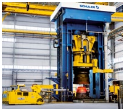
Hydraulic dual forging press with 2 × 140,000 kN press force.
