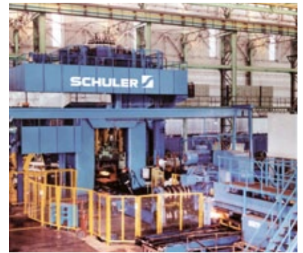
Screw press with direct drive type PZS 900f in operation.
