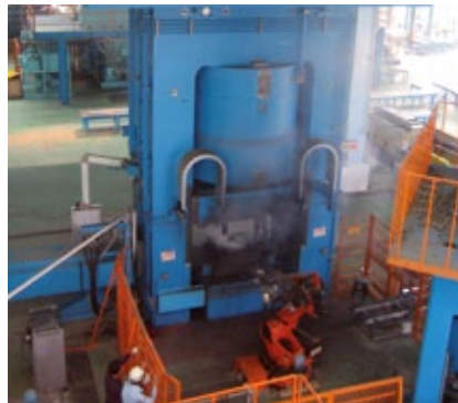
Hydraulic press with 70,000 kN press capacity in production.
