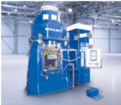
Linear hammer with ServoDirect Technology.
