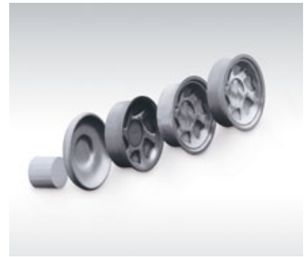
Tool sequence for car aluminum wheels.
