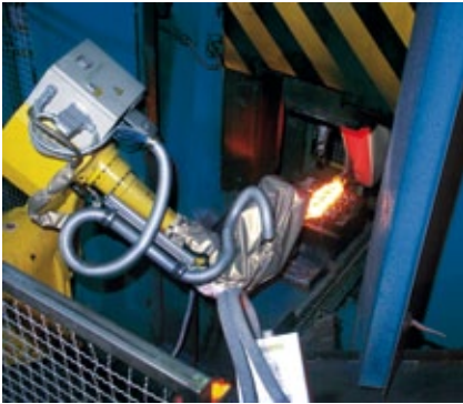
Parts transport and forging using two robots.
