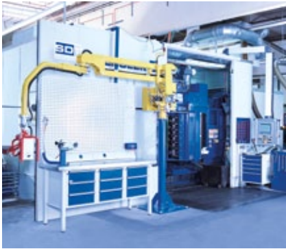
FormMaster with pneumatically supported die change system.
