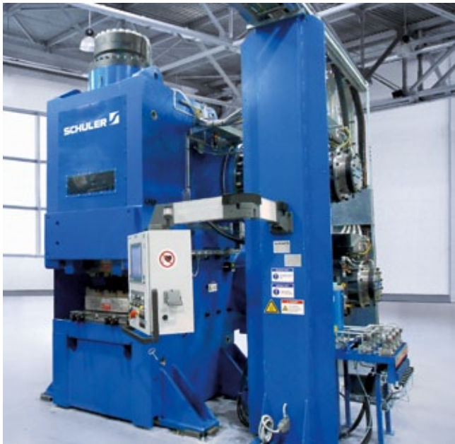
Upsetter with ServoDirect Technology in production.
