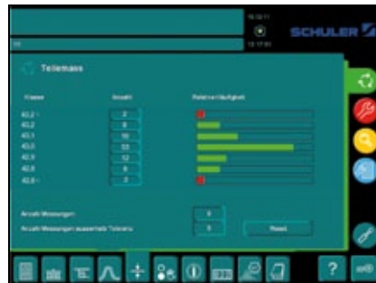
Thickness measurement including Gaussian standard distribution curve.
