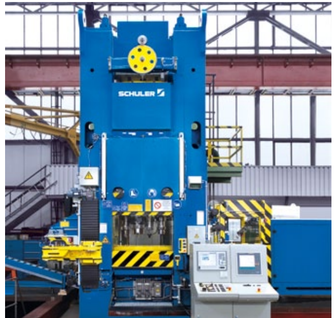
Knuckle joint press with 6,300 kN press force.
