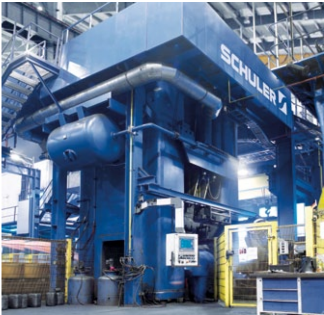
Screw press with direct drive type PZS 900f for manufacturing heavy forgings.
