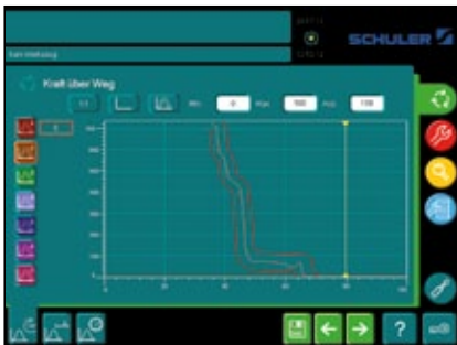
Monitoring of the force/motion profile with envelope curve.
