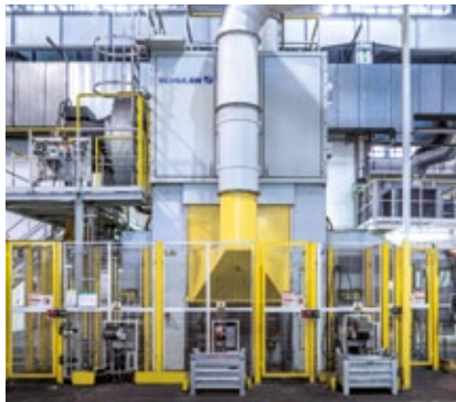
Crank press PK 1600 with ServoDirect technology.
