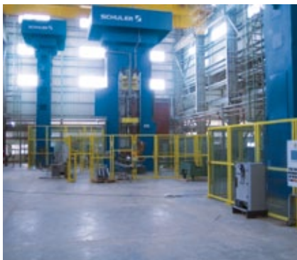
Line for manufacturing CNG gas cylinder tanks from blanks.
