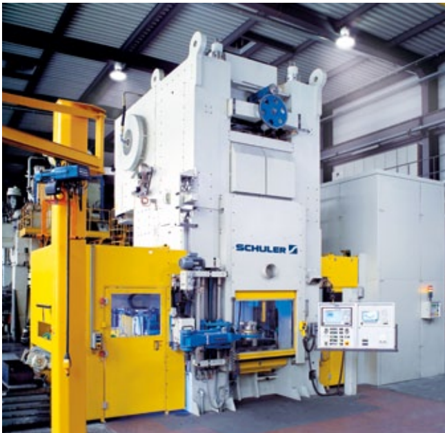
Knuckle joint press with automatic feed from the right, NC transfer system and finished part output.
