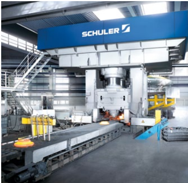
Multi-station hydraulic ring blank press with 35,000 kN press force.
