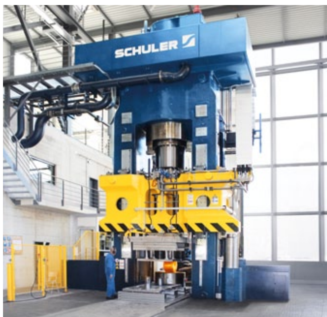
Hydraulic forging press with EHF (Efficient Hydraulic Forming). Energy saving of 60%.
