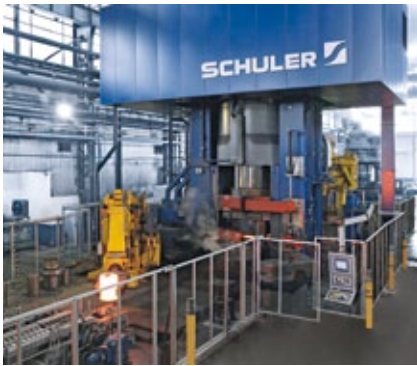
Hydraulic press for forging railway wheels.
