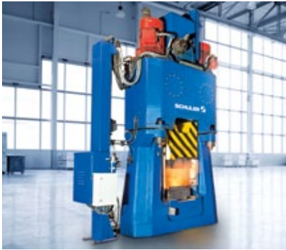
Down stroking hammer with oil hydraulic drive.
