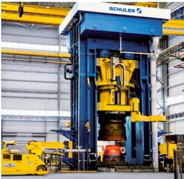
Hydraulic forging press with 140,000 kN press force.
