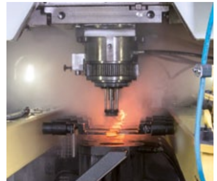
Annealing forging part in the die.
