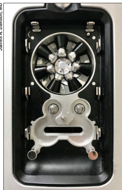
Centurion peristaltic pump, with seven spring-loaded rollers and torsional rotary vent valves.
