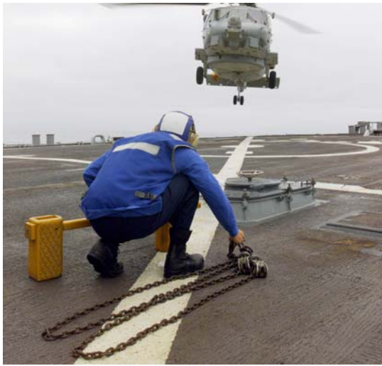
Figure 7 –Deck restraint systems –Traditional chock and chains and RAST (seen beneath helicopter) (www.navy.mil)
