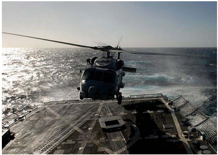
Figure 7 –Deck restraint systems –Traditional chock and chains and RAST (seen beneath helicopter) (www.navy.mil)
