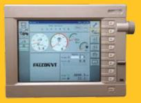
The optional ATS terminal with Falcon™ software is connected to the vehicle's systems via the CAN-BUS network. All information and commands, from application rates to data logging, are shown on the display.
