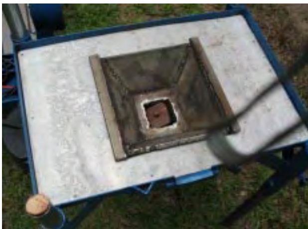
Figure 8: Forge pot & clinker breaker
