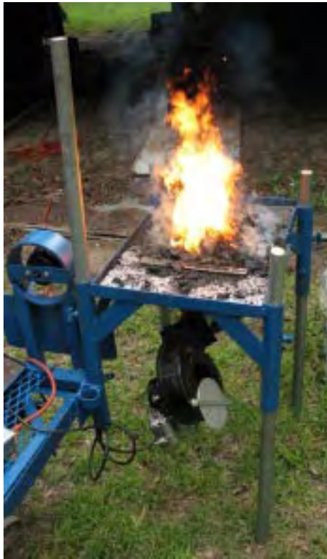
Figure 11: Forge with Fasco blower
