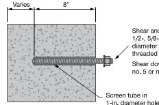
Shear anchor 1/2-, 5/8- or 3/4-in. / diameter ASTM A307 threaded rod Shear dowel no. 4, no. 5 or no. 6 rebar
