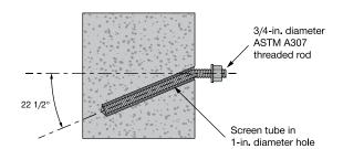
Table 14 - Hilti HIT-HY 70 allowable adhesive bond loads for threaded rods in hollow core concrete panels<sup>1,4,5,6,7</sup>
