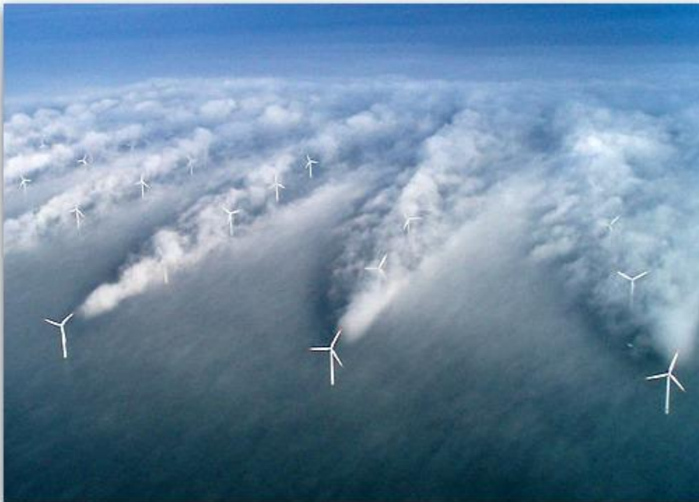
Figure 12: Turbine wake (turbulence) at Horns Rev offshore wind farm
