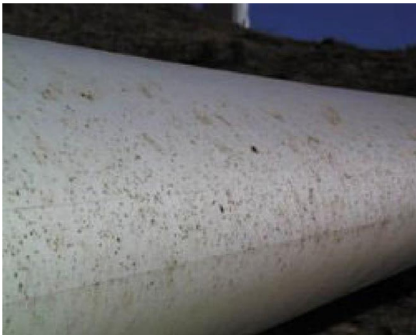
Figure 15: Rotor blade fouling due to insects.
