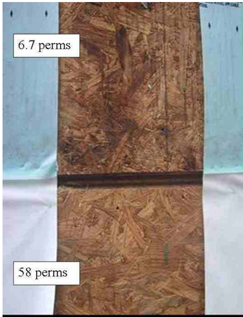
Figure 6 Overlap area between the high- and low-permeability housewraps.
