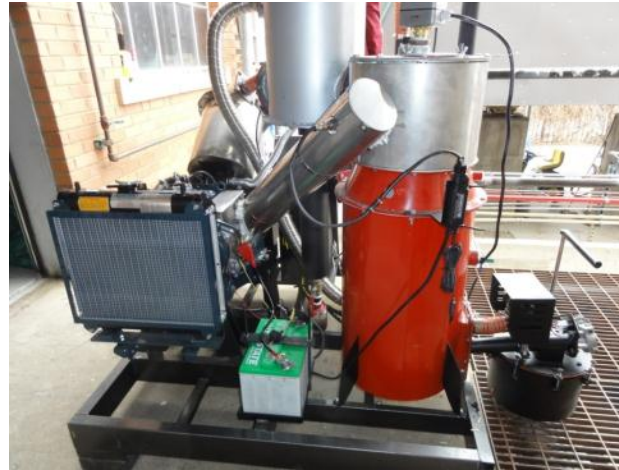
Engine Exhaust Pyrolyzes Chips
