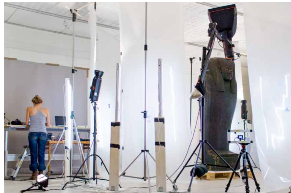
Neswaiu's outer coffin is set up for a photogrammetry session at the studio in Norrköping. Using the cloud-based software Autodesk Recap, the multitude of images from the session is used to generate a complete 3D model of the coffin.
