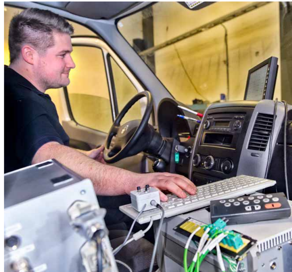
After friction and noise testing, the materials are mounted on a vehicle. Testing is carried out in various locations and several test tracks in Europe and North America, including the Stelvio, Grossglockner and Mojacar.
