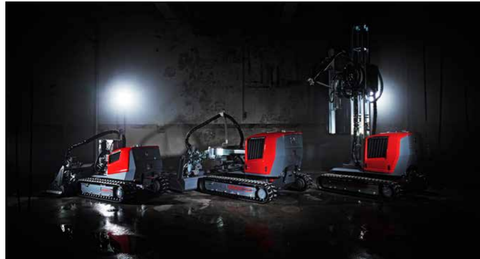
Aquajet's hydrodemolition robots are versatile and made for tough use. Left to right Aqua Cutter 410A for light work, Aqua Cutter 710H for horizontal work and Aqua Cutter 710V for all applications. Images: Aquajet Systems.
