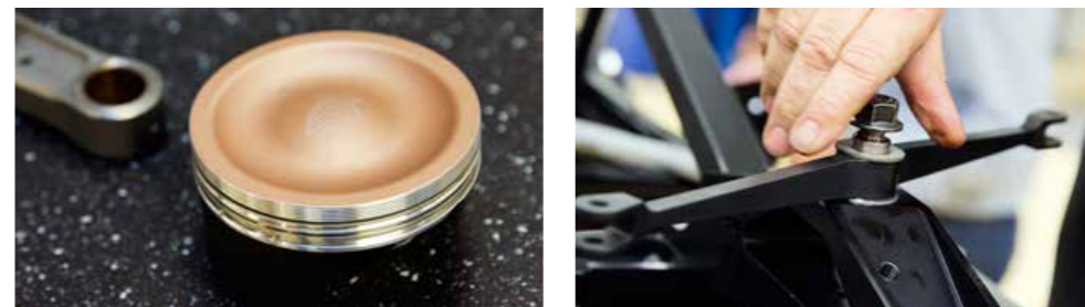
Every part tailor made and handled with the utmost care – left, the superlight forged pistons, right, assembly of body parts.
