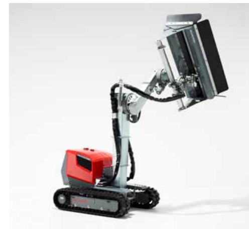
Above and below: Sturdy extensions for the robots provide the range necessary for difficult tasks out of the ordinary reach.
