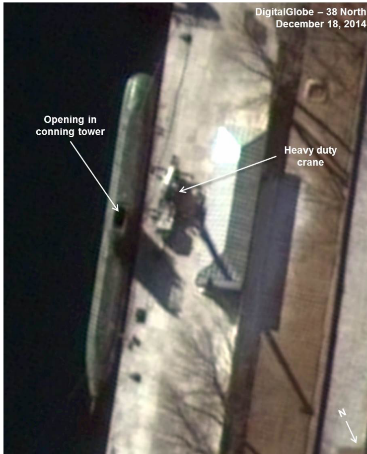
Figure 12: The new Sinpo-class submarine with an opening in the conning tower that may house 1-2 small vertical launch tubes.
