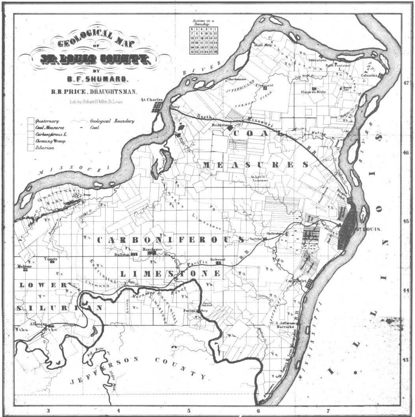
Figure 7. The Geological Map of St. Louis County, published in 1855 with the First and Second Annual Reports, was one of the first geologic maps made by the Missouri Geological Survey, founded in 1853. The immediate St. Louis City area is underlain by St. Louis Limestone (part of the "Carboniferous Limestone"); in places it is overlain by a thin veneer of Pennsylvanian ("Coal Measures") strata.
