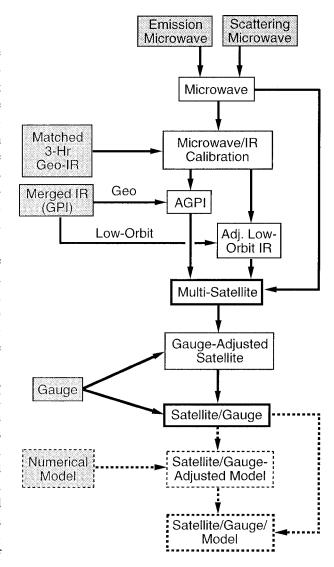
Fig. 1. Flow chart of satellite-gauge-model precipitation combination technique.
