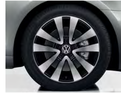
'Seattle Shadow' 7J x 17 light alloy wheels with 225/45 R17 tyres. Standard on GTD models.
