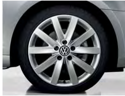
'Porto' 7J x 17 light alloy wheels with 225/45 R17 tyres. Standard on GT models.
