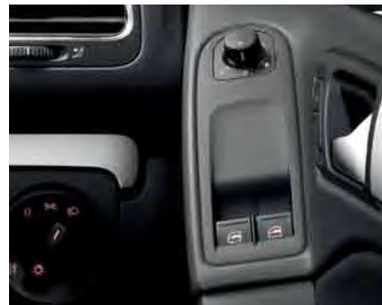
Controls for the electric front windows, including one-touch opening and closing facility, and the electrically heated and adjustable door mirror switch are conveniently located in the driver's door.
