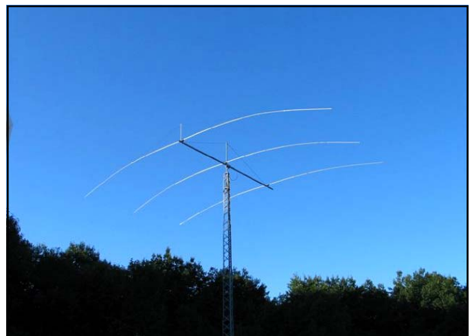
Here's the finished 30m beam, ready for DX action!
